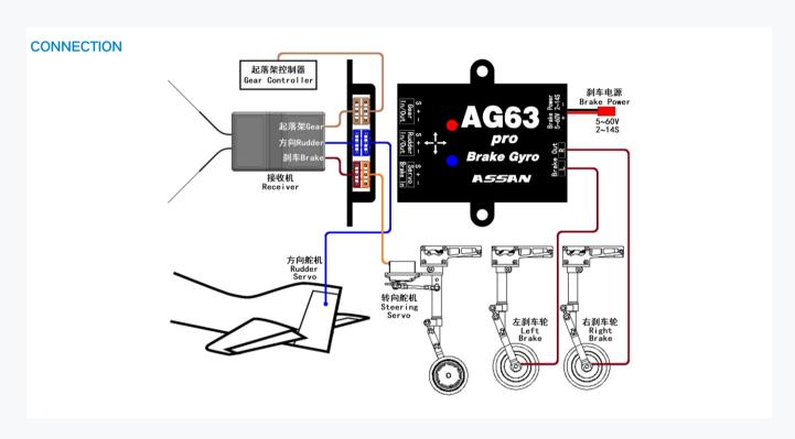
The power supply for the AG63pro gyro is provided by the Rudder channel of the receiver. Power on the receiver and the AG63pro gyro will work. The power input from the brake power plug of the AG63pro gyro is only used to drive the brakes.
